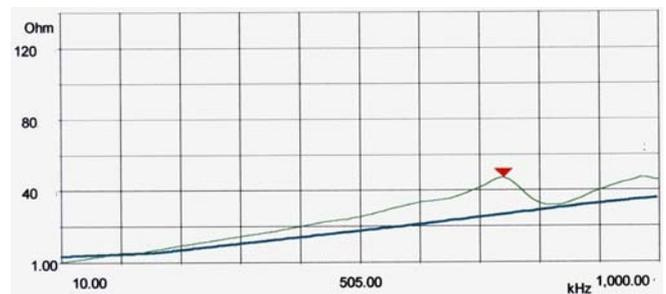
Figure 4. Measurement result for the wound bonding conductor
