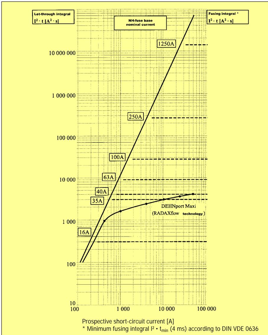
Figure 5: Selectivity peak current with several back-up fuses and DEHNport® Maxi
