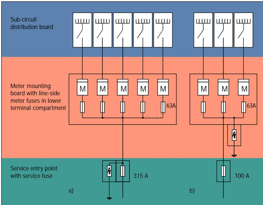
Figure 2: Suggested application of lightning current arresters in main distribution systems with line-side meter fuses
