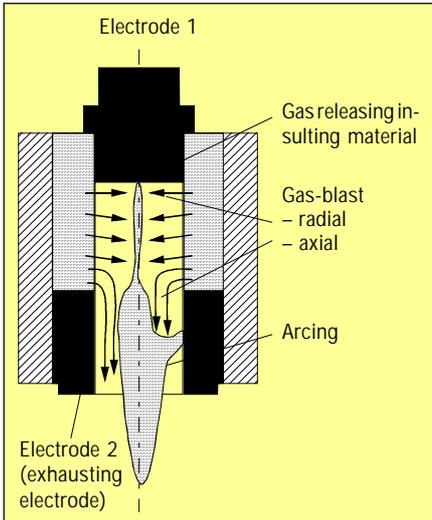
**Figure 3:** Function diagram of an arc blast radially and axially (RADAXflow technology)
