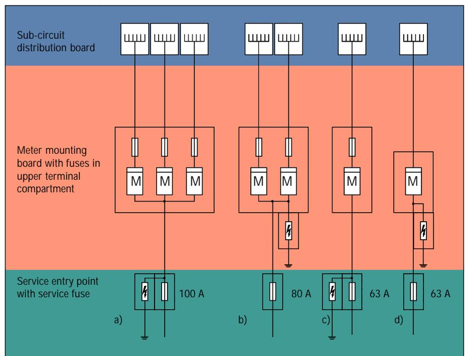
Figure 1: Suggested application of lightning current arresters in main distribution systems without line-side meter fuses
