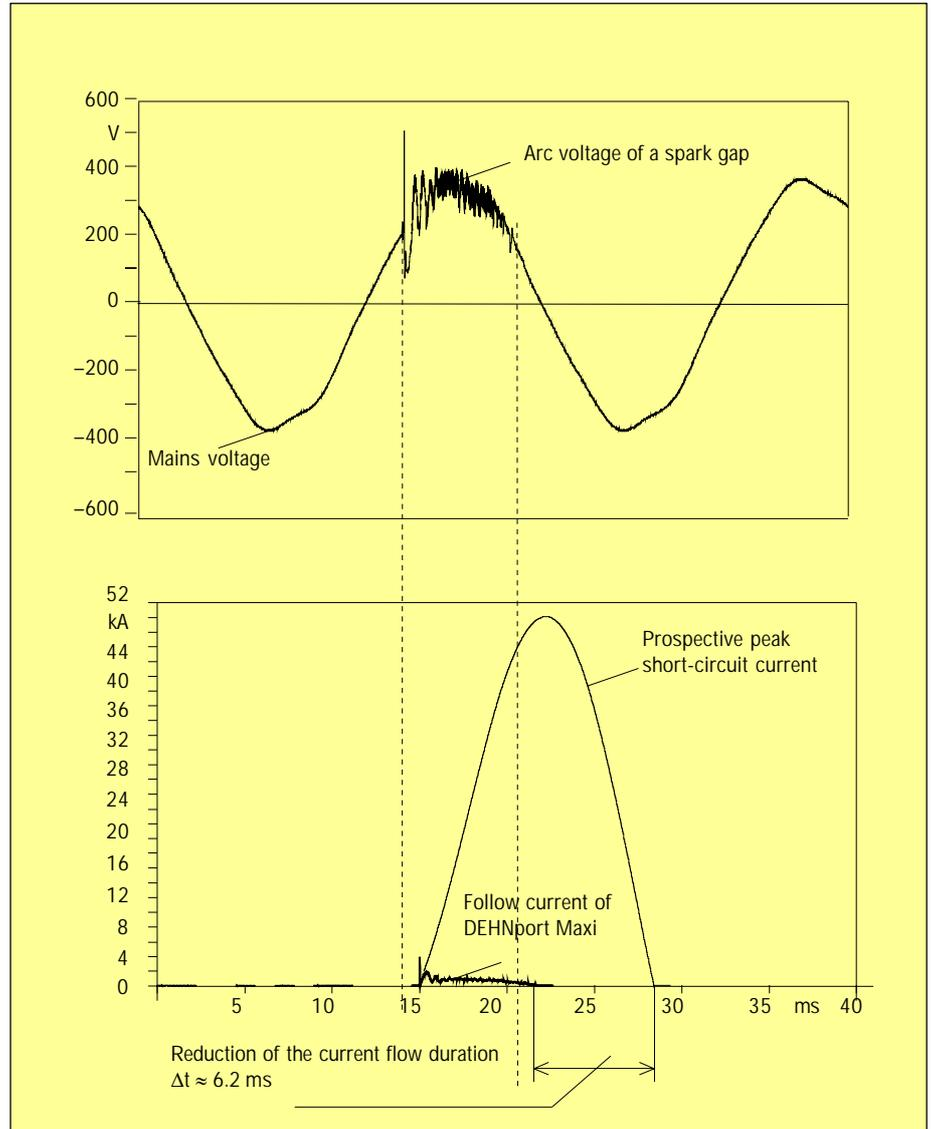
**Figure 4:** Interruption of the short-circuit current using the RADAXflow technology (DEHNport® Maxi)
